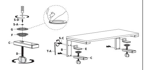
Slide shelf assembly onto desk surface. Tighten Clamp Screw (D) to secure.
