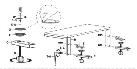
Slide shelf assembly onto desk surface. Tighten Clamp Screw (D) to secure.
